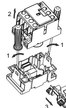
Unscrew pos. 1. Lift the upper part pos.2. Replace the coil pos.3.
