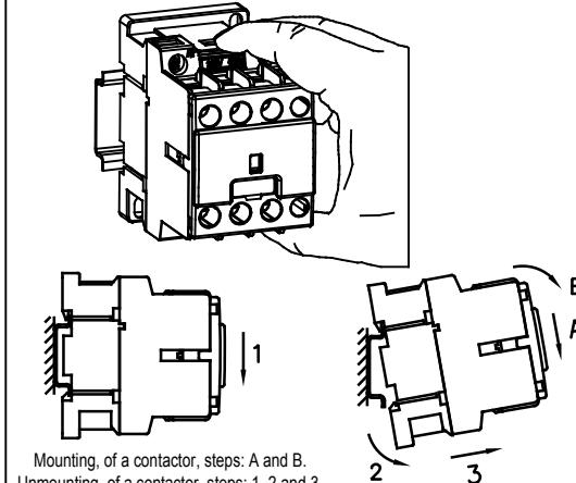
Mounting, of a contactor, steps: A and B.
