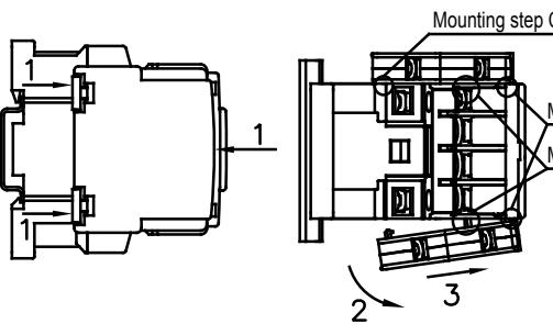
Mounting, of an auxiliary block, steps:
