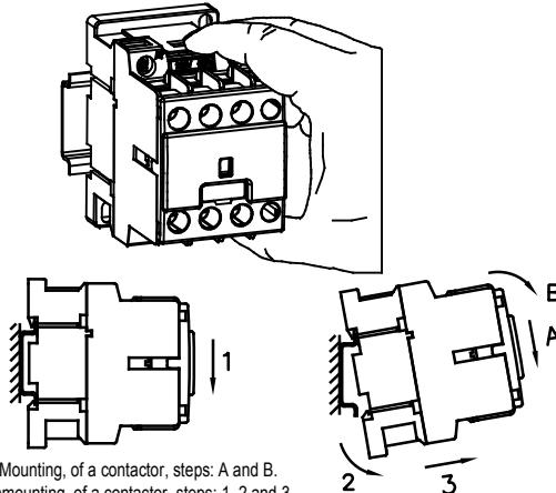
Mounting, of a contactor, steps: A and B.
